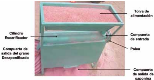
Photograph 4.3. Technical characteristics of the small-scale quinoa processing unit
